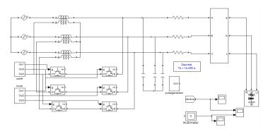
Fig. 5.2. The proposed series-shunt threephase DVR using three-phase PWM ac-ac converter.
