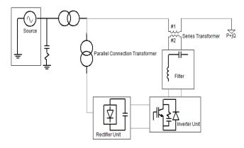
Fig. 2.4 Series ans Parallel Connection Block DVR
