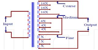
Fig. 3.1 Changing Switch Arrangement in offload
