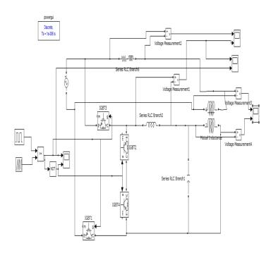
Fig.4.2 . The DVR system with a buck ac-ac converter.
