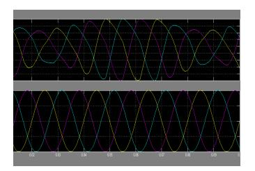
Fig. 5.6. The simulated waveforms when voltage swell occurs, (top) three-phase input voltages, *vsa*, *vsb*, *vsc* with 30% swell, (bottom) threephase .load voltages, *voa*, *vob*, *voc*.
