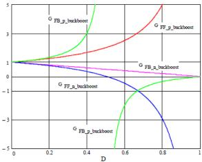
Fig. 4. 1 The overall voltage gains when employing (upper) buck, (Middle) boost, (lower) buck-boost converters.
