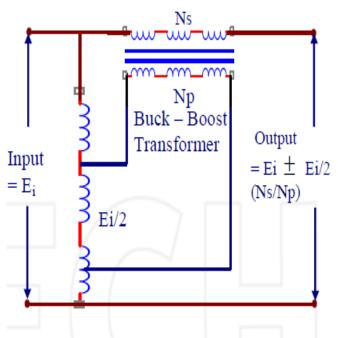
Fig. 3.2 Voltage control by combination of a Buck-Boost transformer and a variac
