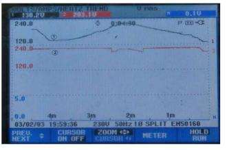
Fig. 5.8 RMS value Voltage wave form.
