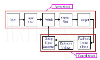
Fig. 2.1 shows the system configuration of the proposed Ac-chopper converters.
