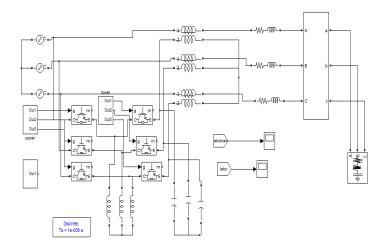
Fig. 5.5. The shunt-series three-phase DVR using three-phase PWM buck-boost ac-ac converter.
