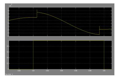
Fig. 5.4. The simulated waveforms when voltage sag occurs, (upper) error voltage, ve, (bottom)  $u_{ty}$  ratio, D.
